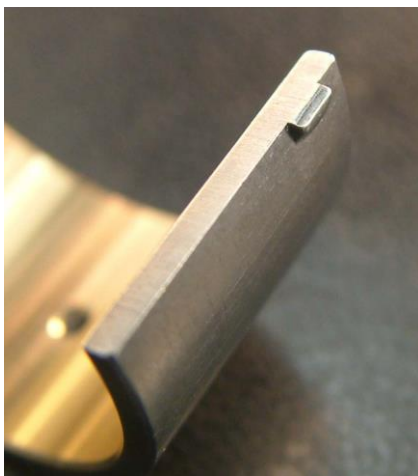
The racing notch allows an uninterrupted joint face
