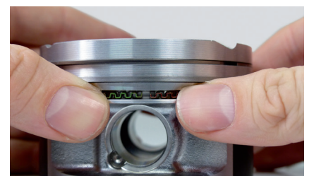
Figure 3: Both color markings on the rails must be visible.
