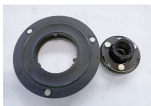
Figure 1 : Protection anti-surcharge déclenchée
