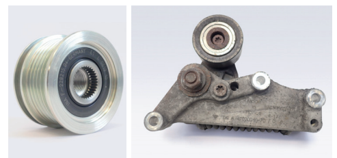
Figure 3: Always check alternator freewheel clutch and belt tension damper.
