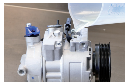
Figure 3: An R134a compressor filled with PAG 46 oil can also be topped off with PAO 68.
