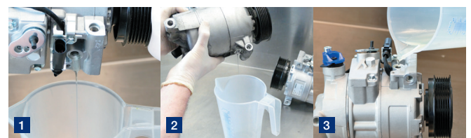
Figure 2: 1. Drain all of the oil from the new compressor. 2. Drain the oil from the old compressor and measure the quantity. 3. Refill the new compressor with a reduced quantity of fresh oil.
