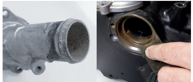
Figure 3: Clean any corroded areas thoroughly prior to assembly.
