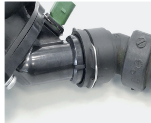
Figure 1: Quick lock on the thermostat housing
