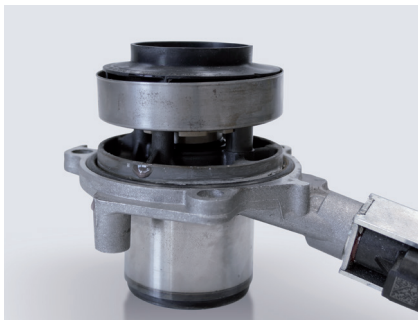
Figure 1: Controlled coolant pump with jammed sliding shroud (no coolant circulation)
