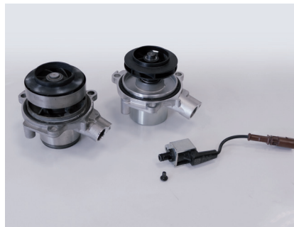
Figure 2: The actuator must be detached from the controlled pump, then reattached to the new pump.
