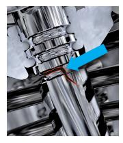
Figure 2: Valve fracture at the lowest groove
