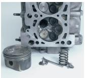
Figure 5: Typical damage scenario after a valve has torn off
