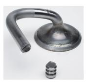
Figure 4: Broken valve
