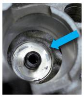
Figure 3: Pressure marks in the cylinder head
