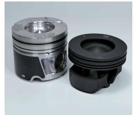
Figure 2: The diameter is measured at a right angle to the pin axis on the skirt.
