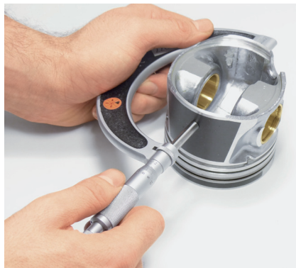
Figure 2: The diameter is measured at a right angle to the pin axis on the skirt.
