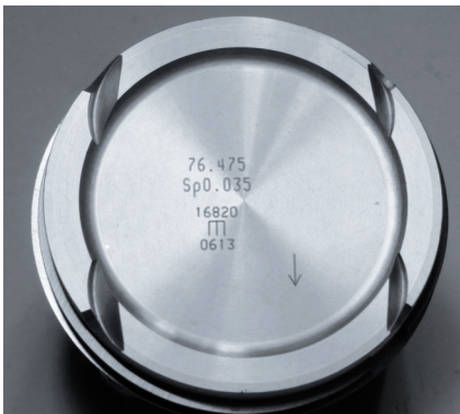
Figure 1: Information on the piston crown—diameter, installation clearance, and installation direction (arrow)
