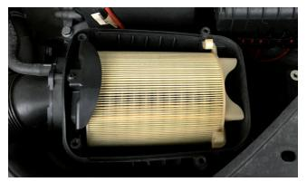
Figure 1: Comparable air filter element, installed.
