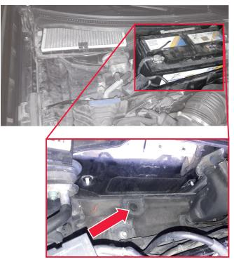
Figure 2: Water drain (indicated by arrow) below the battery in the water tank
