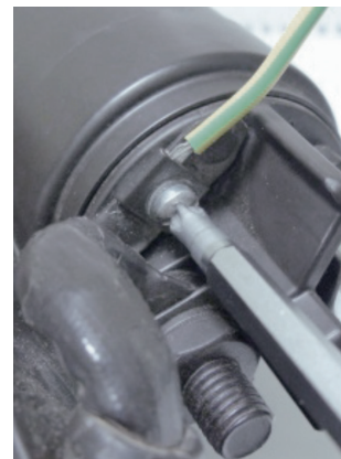
Figure 3: Cable attached to clamp 50 of the solenoid
