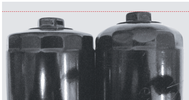
Figure 3: Oil filters, side-by-side comparison—left: normal, right: deformed
