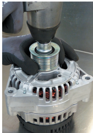
Figure 2: Impact drivers are only used to loosen the pulley, NEVER to tighten it!
