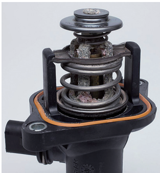
Figure 1: Obvious signs of corrosion on a map-controlled thermostat (Type TM).
