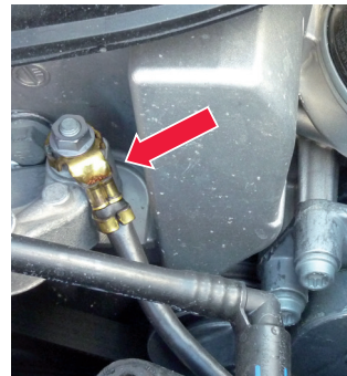
Figure 3: Check the earthing cable to ensure it is properly connected and free of damage.
