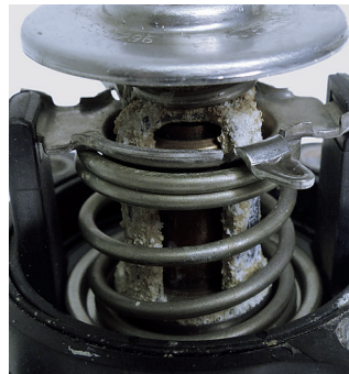
Figure 2: The aluminium has been completely eaten away due to the use of non-approved coolant additives.
