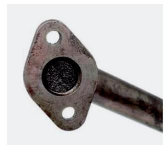
Figure 4: Carbonised oil return line
