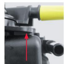
Then, press the lower edge of the heater against the filter so that it can lock into the lower clip. Check that the part is correctly fitted by attempting to push it forwards in the direction of the mounting hole.
