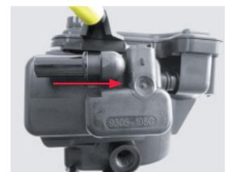
Removal: press the left-hand side of the lower clip downwards and push the lower edge of the heater forwards. Then pull the heater away from the filter and out of the mounting hole—in the opposite direction of installation.
