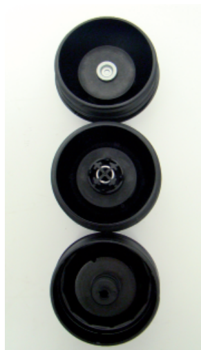
Figure 2: Oil filter, inner view: three different threaded covers
