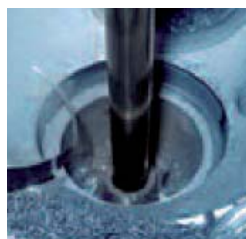
Figure 2: After milling a remainder of the insert can be seen.
