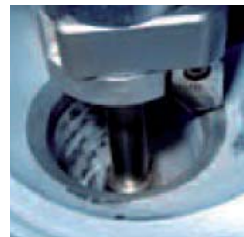
Figure 3: The milling head for machining the seat of the valve seat insert.
