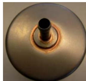
Figure 2 and 3: Fuel filter with arrears of brazing
