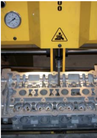
Figure 1: Pressing out of the valve guide
