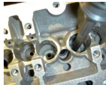
Figure 2: Pressing in of the valve guide
