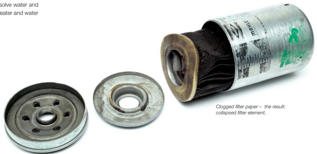
*Clogged filter paper – the result: collapsed filter element.*
