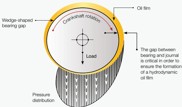
Schematic diagram of the loads in a hydrodynamic bearing.
