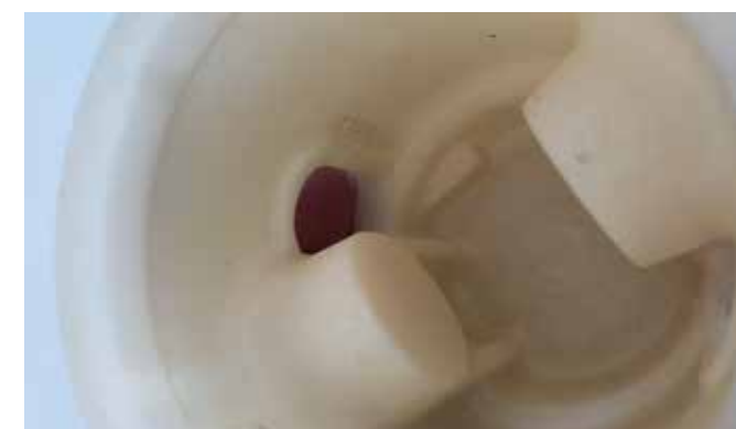
A look inside the printed blank (still in plastic) of a two-stroke piston for an Auto Union 1000 S
