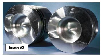
Image #3 shows the piston crowns of these same two pistons. Notice how two pistons with the same casting number can have distinctively different crown designs. The piston on the left (OE# 154-8087) has two valve pockets and piston on the right (OE#107-3565) has only one valve pocket.
