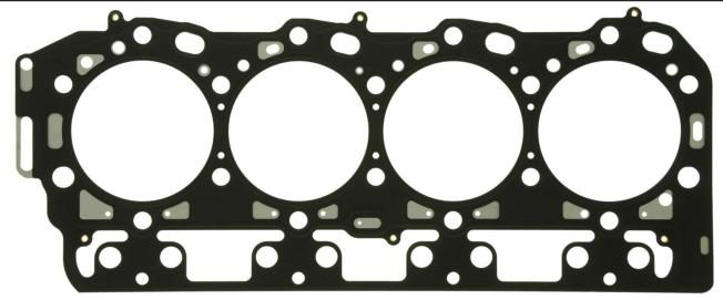
**MAHLE Original Part # 54597**: a patented stopper design featuring concentric waves around the combustion chamber (in the spring steel active layer) allowing the head gasket to adapt to varying loads and pressures.
