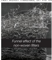
with thicknesses in the micron range: the finer the fibers, the better the separation. The non-woven materials are applied in layers in which the density and fineness of the fibers increase from the dirt side to the clean side. This so-called funnel effect allows efficiencies of up to 99.9 percent with low flow resistance at the same time.
