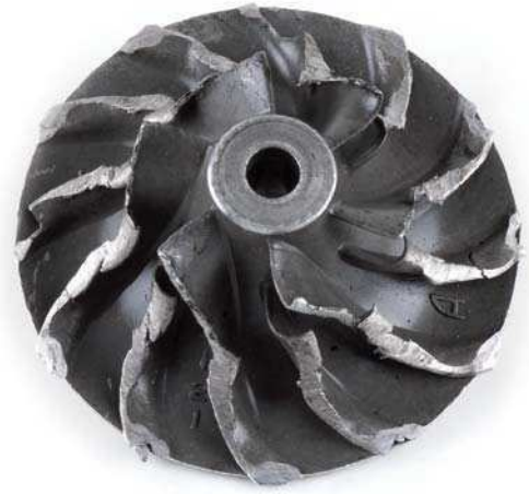
Fig. 1 Impeller after contact with housing
