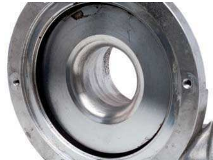
Fig. 2 Contact marks in the compressor housing
