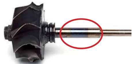
Fig. 3 Discoloration of the shaft shank
