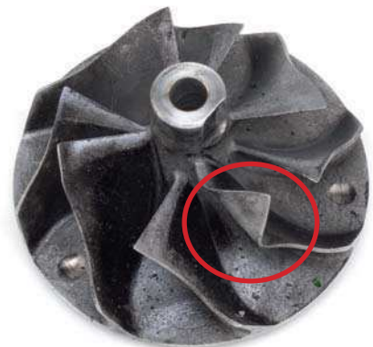
Fig. 4 Only one vane of the impeller damaged
