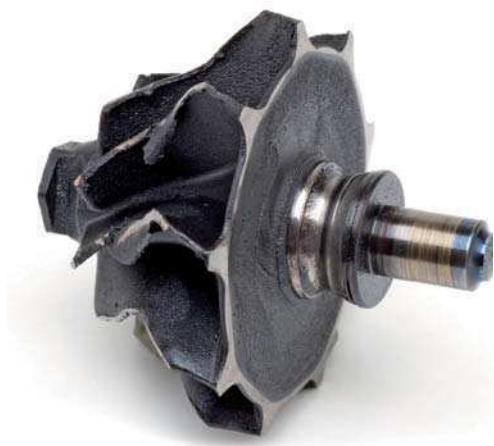
Fig. 5 Broken shaft shank
