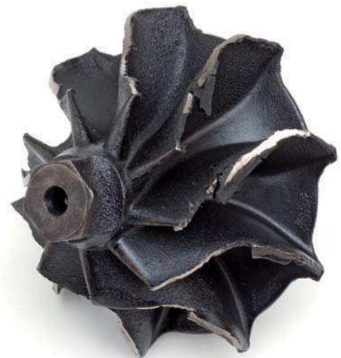
Fig. 2 Turbine wheel after contact with housing
