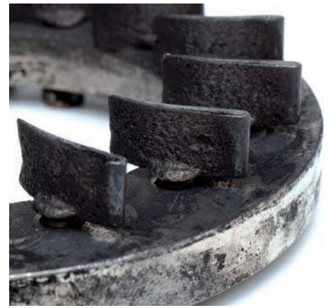
Fig. 1 Damaged air guide plates of the VTG unit
