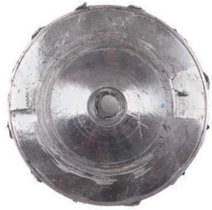
Fig. 1 Dents on the rear of the impeller
