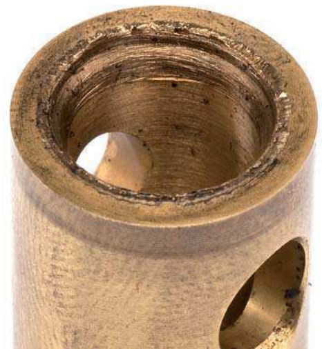
Fig. 1 Grooves in the radial bearing
