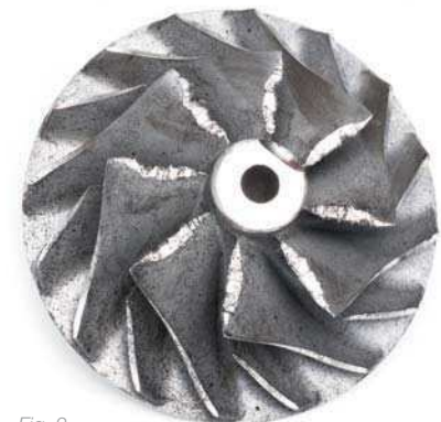
Fig. 2 Impeller damaged by foreign substances
