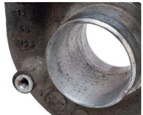
Fig. 3 Foreign substance impact in the intake passage of the compressor housing
