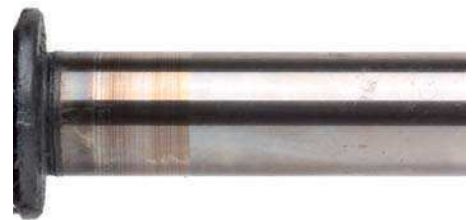
Fig. 4 Bearing material fused onto the shaft
