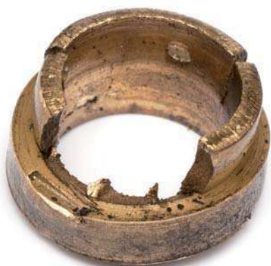
Fig. 7 Broken radial bearing
