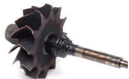
Fig. 3 Carbonised oil on the turbine side
