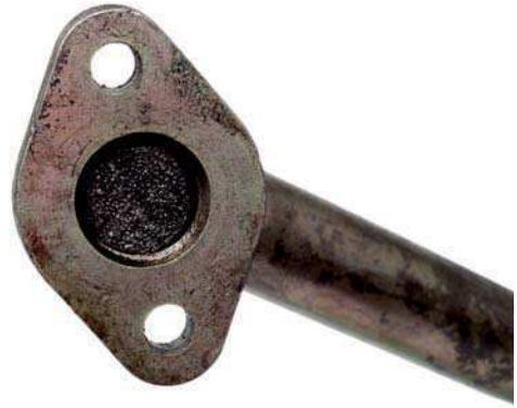
Fig. 1 Carbonised oil return line
