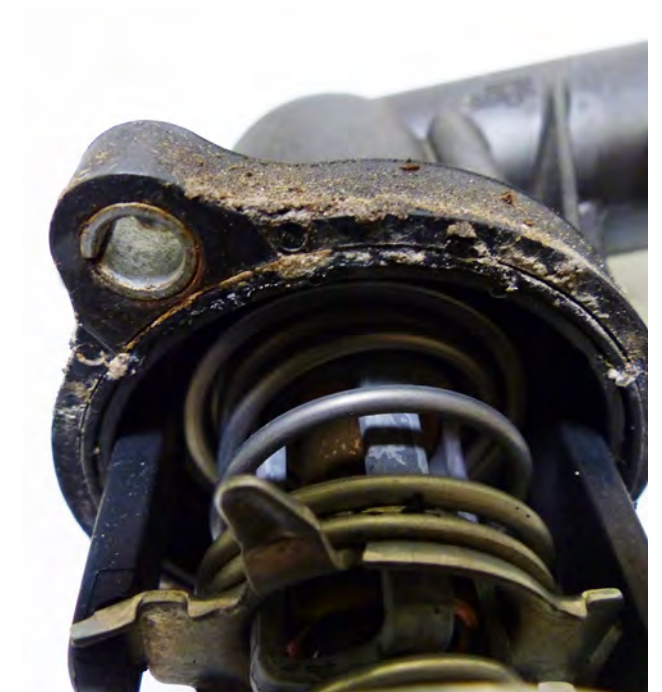
Fig. 2: Seal damaged by additional sealing compound
