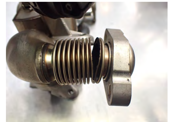
Fig. 2: Crack in the flexible pipe from the EGR cooler
