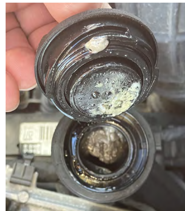
Fig. 2: Oil-in-water emulsion on the oil filler cap and in the oil filler neck
