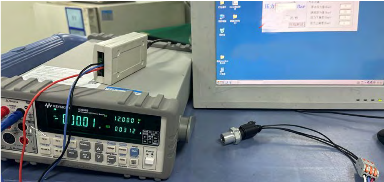
Fig. 4: Testing a pressure switch in the laboratory
