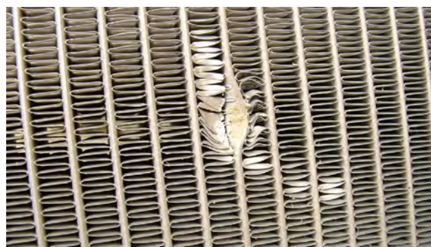
Fig. 3: Stone chipping on the radiator
