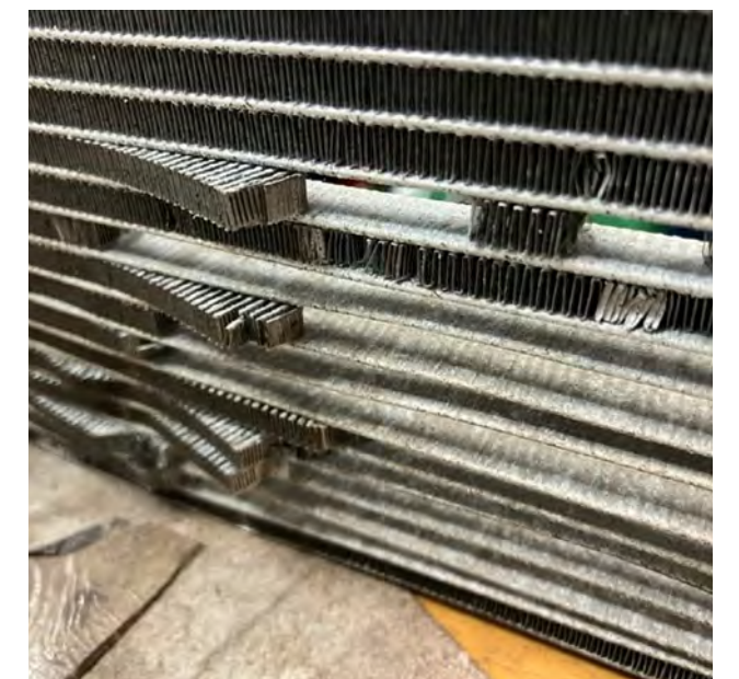
Fig. 2: Corroded cooling fins
