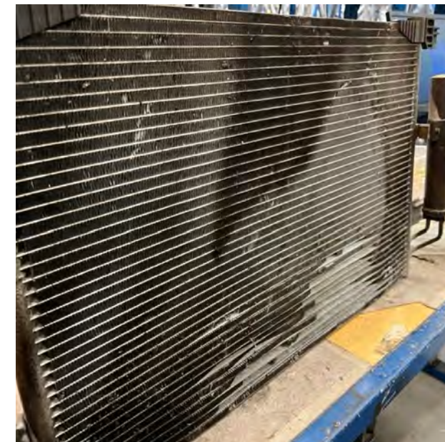
Fig. 1: Corrosion on the condenser
