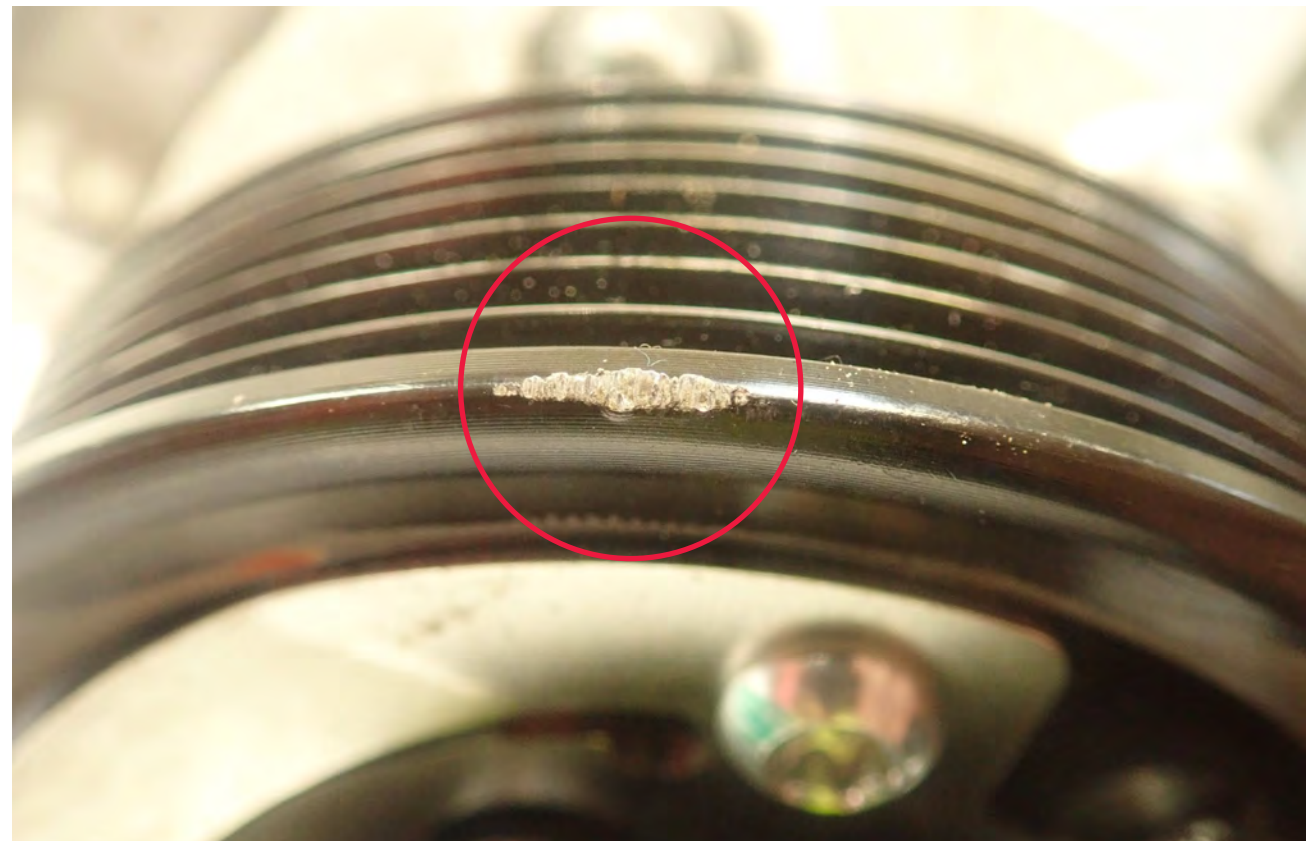
Fig. 1: Damaged belt pulley
