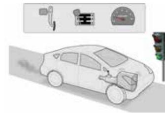
Press the clutch, engage the gear—the engine starts automatically.
