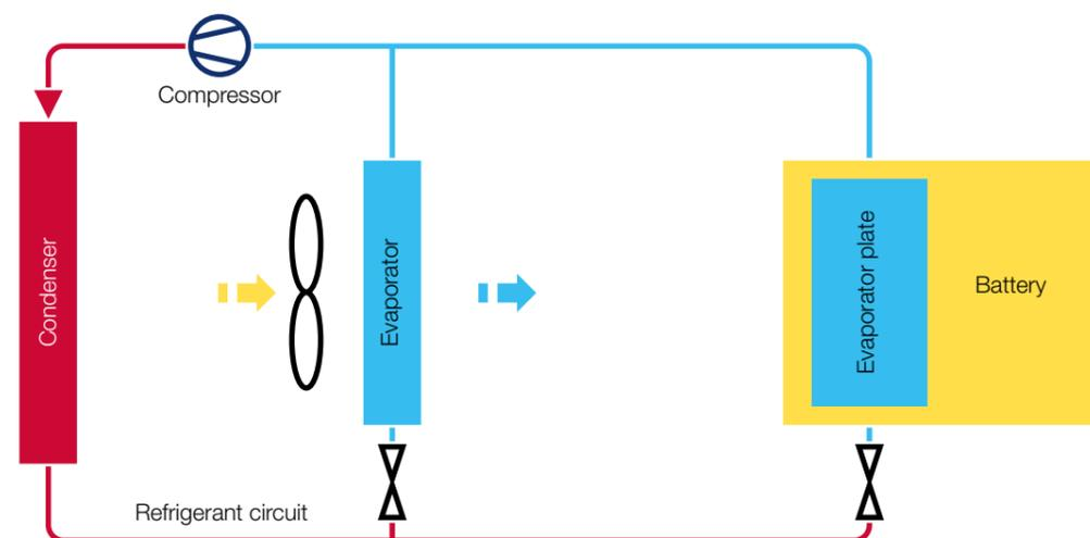
A special evaporator plate inside the battery cell is connected to the air conditioning system in the vehicle. This is done using what is known as the splitting process on the high-pressure and low-pressure side via pipelines and an expansion valve. This means that the interior evaporator and the evaporator plate of the battery, which works like a conventional evaporator, are connected to the same circuit.
