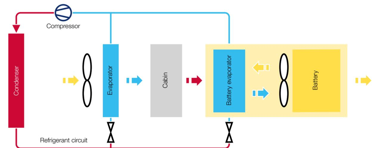
Air is drawn in from the air-conditioned vehicle cabin and used to cool the battery. The cool air drawn in from the cabin has
