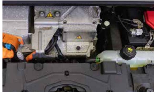
High-voltage components in the engine compartment
