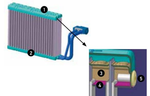
Schematic diagram of storage evaporator: (1) evaporator core 40 mm deep, (2) storage core 15 mm deep, (3) refrigerant, (4) latent medium, (5) blind rivet
