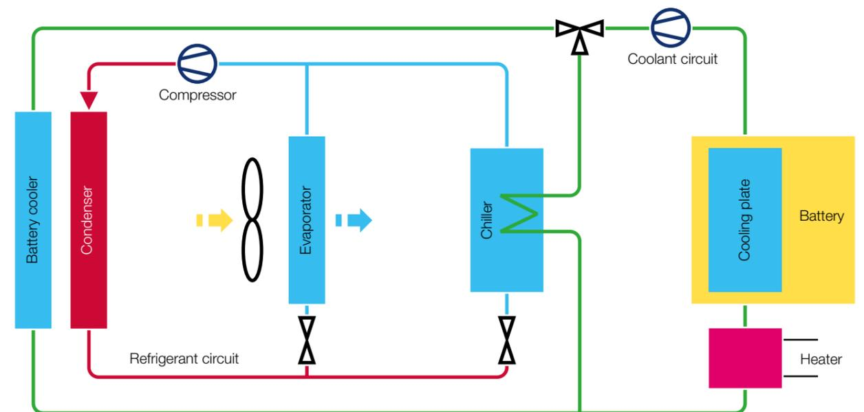
The correct temperature plays a key role for batteries with higher capacities. Therefore, at very low temperatures, additional heating of the battery is required to bring it to the ideal temperature range. This is the only way to achieve a satisfactory cruising range when in “electric driving” mode.
