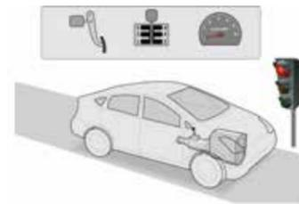
The vehicle comes to a stop—the engine switches off automatically.
