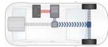
Electric driving—driven solely by the electric motor
