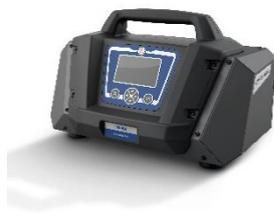
Also available as a standalone tool: The MAHLE PMU 400 for measuring particles from the tail pipe.
